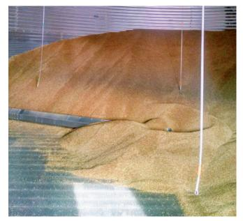
These sensor cables inside a wheat bin at Arrow K Farms assess temperature and moisture. The information is reported and recorded electronically through a system developed by IntelliFarms. Then, the Kessels can open an app on a mobile phone or personal computer, and learn the findings — and even change the fan settings.
